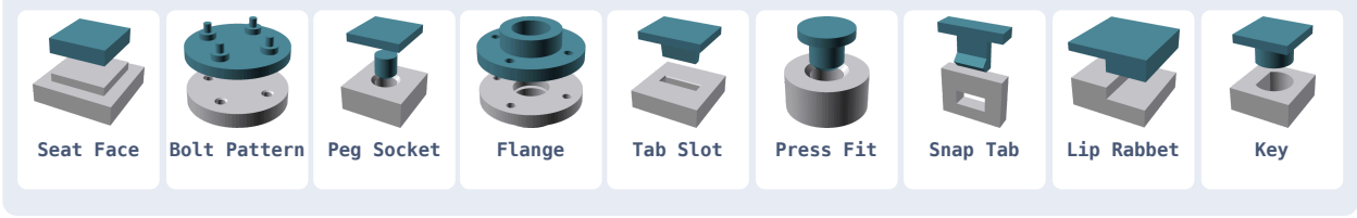
Figure 4. The mate library. The nine static mating features a part may declare, each rendered from the compiler macros the build emits. Teal is the male half added to the new part and grey the female half cut from its partner; both derive from one shared nominal dimension and a signed fit offset.
